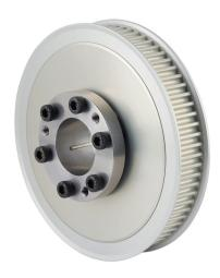
Sung-Il Machinery timing pulley, aluminum, 5mm 5M pitch, 72 tooth, 4.511in pitch diameter, 1-1/8in bore, no hub with flanges. For use with 15mm wide belt. QD bushing included.
