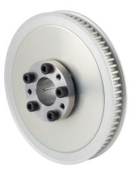
Sung-Il Machinery timing pulley, aluminum, 5mm 5M pitch, 72 tooth, 4.511in pitch diameter, 7/8in bore, no hub with flanges. For use with 9mm wide belt. QD bushing included.
