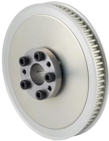
Sung-II Machinery timing pulley, aluminum, 5mm 5M pitch, 72 tooth, 4.511in pitch diameter, 3/4in bore, no hub with flanges. For use with 9mm wide belt. QD bushing included.
