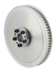
Sung-Il Machinery timing pulley, aluminum, 5mm 5M pitch, 72 tooth, 4.511in pitch diameter, 5/8in bore, no hub with flanges. For use with 9mm wide belt. QD bushing included.
