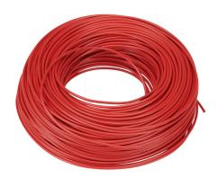
LUTZE HAR H05V-K hook-up wire, single conductor, 19 AWG (0.75mm2), 24-stranded, tinned copper, PVC conductor insulation material, red, 300/500V (H05V2-K), 600V (MTW), 328ft carton.
