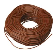
LUTZE HAR H05V-K hook-up wire, single conductor, 19 AWG (0.75mm2), 24-stranded, tinned copper, PVC conductor insulation material, brown, 300/500V (H05V2-K), 600V (MTW), 328ft carton.
