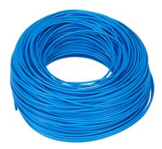
LUTZE HAR H05V-K hook-up wire, single conductor, 19 AWG (0.75mm2), 24-stranded, tinned copper, PVC conductor insulation material, blue, 300/500V (H05V2-K), 600V (MTW), 328ft carton.
