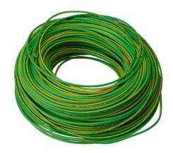
LUTZE HAR H05V-K hook-up wire, single conductor, 19 AWG (0.75mm2), 24-stranded, tinned copper, PVC conductor insulation material, green/yellow, 300/500V (H05V2-K), 600V (MTW), 328ft carton.
