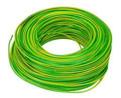
LUTZE HAR H05V-K hook-up wire, single conductor, 18 AWG (1.0mm2), 32-stranded, tinned copper, PVC conductor insulation material, green/yellow, 300/500V (H05V2-K), 600V (MTW), 328ft carton.
