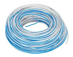
LUTZE HAR H07V-K hook-up wire, single conductor, 16 AWG (1.50mm2), 30-stranded, tinned copper, PVC conductor insulation material, white/blue, 450/750V (H07V2-K), 600V (MTW), 328ft carton.
