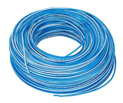
LUTZE HAR H07V-K hook-up wire, single conductor, 16 AWG (1.50mm2), 30-stranded, tinned copper, PVC conductor insulation material, blue/white, 450/750V (H07V2-K), 600V (MTW), 328ft carton.
