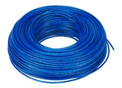
LUTZE HAR H07V-K hook-up wire, single conductor, 16 AWG (1.50mm2), 30-stranded, tinned copper, PVC conductor insulation material, dark blue, 450/750V (H07V2-K), 600V (MTW), 328ft carton.
