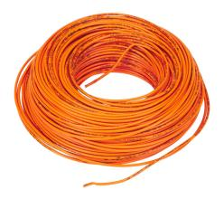
LUTZE HAR H07V-K hook-up wire, single conductor, 16 AWG (1.50mm2), 30-stranded, tinned copper, PVC conductor insulation material, orange, 450/750V (H07V2-K), 600V (MTW), 328ft carton.
