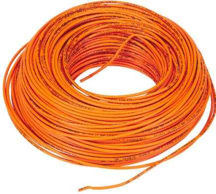
LUTZE HAR H07V-K hook-up wire, single conductor, 16 AWG (1.50mm<sup>2</sup>), 30-stranded, tinned copper, PVC conductor insulation material, orange, 450/750V (H07V2-K), 600V (MTW), 328ft carton.
