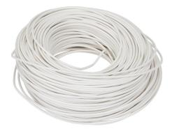
LUTZE HAR H07V-K hook-up wire, single conductor, 16 AWG (1.50mm2), 30-stranded, tinned copper, PVC conductor insulation material, white, 450/750V (H07V2-K), 600V (MTW), 328ft carton.
