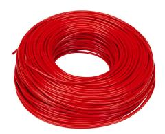
LUTZE HAR H07V-K hook-up wire, single conductor, 16 AWG (1.50mm2), 30-stranded, tinned copper, PVC conductor insulation material, red, 450/750V (H07V2-K), 600V (MTW), 328ft carton.
