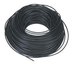
LUTZE HAR H07V-K hook-up wire, single conductor, 16 AWG (1.50mm2), 30-stranded, tinned copper, PVC conductor insulation material, black, 450/750V (H07V2-K), 600V (MTW), 328ft carton.
