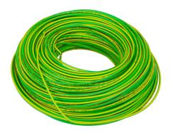
LUTZE HAR H07V-K hook-up wire, single conductor, 16 AWG (1.50mm2), 30-stranded, tinned copper, PVC conductor insulation material, green/yellow, 450/750V (H07V2-K), 600V (MTW), 328ft carton.
