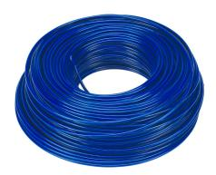
LUTZE HAR H07V-K hook-up wire, single conductor, 14 AWG (2.50mm2), 50-stranded, tinned copper, PVC conductor insulation material, dark blue, 450/750V (H07V2-K), 600V (MTW), 328ft carton.
