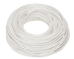
LUTZE HAR H07V-K hook-up wire, single conductor, 14 AWG (2.50mm2), 50-stranded, tinned copper, PVC conductor insulation material, white, 450/750V (H07V2-K), 600V (MTW), 328ft carton.
