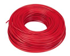
LUTZE HAR H07V-K hook-up wire, single conductor, 14 AWG (2.50mm2), 50-stranded, tinned copper, PVC conductor insulation material, red, 450/750V (H07V2-K), 600V (MTW), 328ft carton.
