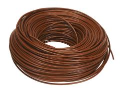
LUTZE HAR H07V-K hook-up wire, single conductor, 14 AWG (2.50mm2), 50-stranded, tinned copper, PVC conductor insulation material, brown, 450/750V (H07V2-K), 600V (MTW), 328ft carton.
