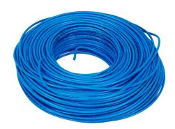
LUTZE HAR H07V-K hook-up wire, single conductor, 14 AWG (2.50mm2), 50-stranded, tinned copper, PVC conductor insulation material, blue, 450/750V (H07V2-K), 600V (MTW), 328ft carton.
