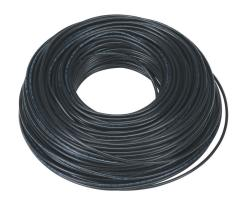
LUTZE HAR H07V-K hook-up wire, single conductor, 14 AWG (2.50mm2), 50-stranded, tinned copper, PVC conductor insulation material, black, 450/750V (H07V2-K), 600V (MTW), 328ft carton.
