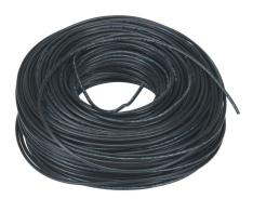
LUTZE HAR H07V-K hook-up wire, single conductor, 12 AWG (4mm2), 56-stranded, tinned copper, PVC conductor insulation material, black, 450/750V (H07V2-K), 600V (MTW), 328ft carton.
