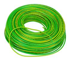
LUTZE HAR H07V-K hook-up wire, single conductor, 12 AWG (4mm2), 56-stranded, tinned copper, PVC conductor insulation material, green/yellow, 450/750V (H07V2-K), 600V (MTW), 328ft carton.
