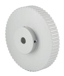
Sung-II Machinery timing pulley, aluminum, 1/5in XL pitch, 60 tooth, 3.82in pitch diameter, 3/8in bore, hub without flanges. For use with 3/8in wide belt.
