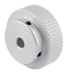
Sung-Il Machinery timing pulley, aluminum, 0.08in MXL pitch, 60 tooth, 1.528in pitch diameter, 1/4in bore, hub without flanges. For use with 1/4in wide belt.
