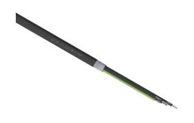
LUTZE Silflex FBP VFD cable, overall foil and braid shielded, 4 conductors (includes ground), 18 AWG, tinned copper, XLPE conductor insulation material, black with white numbers and green/yellow ground, TPE jacket, black, cut to length.
