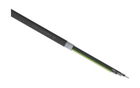
LUTZE Silflex FBP VFD cable, overall foil and braid shielded, 4 conductors (includes ground), 16 AWG, tinned copper, XLPE conductor insulation material, black with white numbers and green/yellow ground, TPE jacket, black, cut to length.
