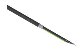
LUTZE Silflex FBP VFD cable, overall foil and braid shielded, 4 conductors (includes ground), 14 AWG, tinned copper, XLPE conductor insulation material, black with white numbers and green/yellow ground, TPE jacket, black, cut to length.
