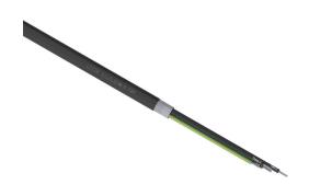
LUTZE Silflex FBP VFD cable, overall foil and braid shielded, 4 conductors (includes ground), 12 AWG, tinned copper, XLPE conductor insulation material, black with white numbers and green/yellow ground, TPE jacket, black, cut to length.
