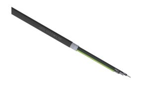
LUTZE Silflex FBP VFD cable, overall foil and braid shielded, 4 conductors (includes ground), 10 AWG, tinned copper, XLPE conductor insulation material, black with white numbers and green/yellow ground, TPE jacket, black, cut to length.
