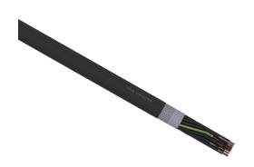
LUTZE Silflex FBP flexible control cable, shielded, 25 conductors (includes ground), 20 AWG, bare copper, polypropylene conductor insulation material, black with white numbers and green/yellow ground, TPE jacket, black, cut to length.
