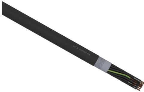
LUTZE Silflex FBP flexible control cable, shielded, 25 conductors (includes ground), 20 AWG, bare copper, polypropylene conductor insulation material, black with white numbers and green/yellow ground, TPE jacket, black, cut to length.
