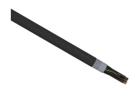
LUTZE Silflex FBP flexible control cable, shielded, 18 conductors (includes ground), 20 AWG, bare copper, polypropylene conductor insulation material, black with white numbers and green/yellow ground, TPE jacket, black, cut to length.
