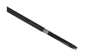
LUTZE Silflex FBP flexible control cable, shielded, 12 conductors (includes ground), 20 AWG, bare copper, polypropylene conductor insulation material, black with white numbers and green/yellow ground, TPE jacket, black, cut to length.
