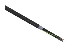
LUTZE Silflex FBP flexible control cable, shielded, 7 conductors (includes ground), 20 AWG, bare copper, polypropylene conductor insulation material, black with white numbers and green/yellow ground, TPE jacket, black, cut to length.
