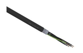
LUTZE Silflex FBP flexible control cable, shielded, 5 conductors (includes ground), 20 AWG, bare copper, polypropylene conductor insulation material, black with white numbers and green/yellow ground, TPE jacket, black, cut to length.
