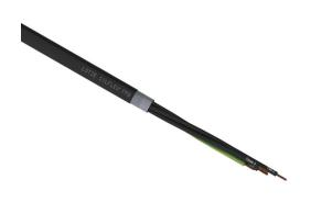
LUTZE Silflex FBP flexible control cable, shielded, 4 conductors (includes ground), 20 AWG, bare copper, polypropylene conductor insulation material, black with white numbers and green/yellow ground, TPE jacket, black, cut to length.
