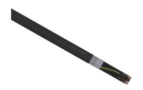
LUTZE Silflex FBP flexible control cable, shielded, 25 conductors (includes ground), 18 AWG, bare copper, polypropylene conductor insulation material, black with white numbers and green/yellow ground, TPE jacket, black, cut to length.
