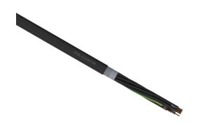
LUTZE Silflex FBP flexible control cable, shielded, 12 conductors (includes ground), 18 AWG, bare copper, polypropylene conductor insulation material, black with white numbers and green/yellow ground, TPE jacket, black, cut to length.
