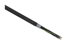
LUTZE Silflex FBP flexible control cable, shielded, 7 conductors (includes ground), 18 AWG, bare copper, polypropylene conductor insulation material, black with white numbers and green/yellow ground, TPE jacket, black, cut to length.
