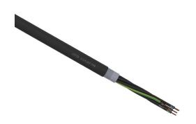
LUTZE Silflex FBP flexible control cable, shielded, 7 conductors (includes ground), 18 AWG, bare copper, polypropylene conductor insulation material, black with white numbers and green/yellow ground, TPE jacket, black, cut to length.
