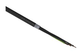
LUTZE Silflex FBP flexible control cable, shielded, 4 conductors (includes ground), 18 AWG, bare copper, polypropylene conductor insulation material, black with white numbers and green/yellow ground, TPE jacket, black, cut to length.
