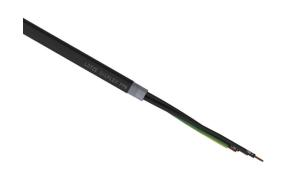
LUTZE Silflex FBP flexible control cable, shielded, 3 conductors (includes ground), 18 AWG, bare copper, polypropylene conductor insulation material, black with white numbers and green/yellow ground, TPE jacket, black, cut to length.
