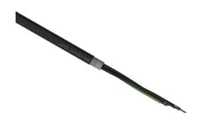
LUTZE Silflex FBP flexible control cable, shielded, 3 conductors (includes ground), 18 AWG, bare copper, polypropylene conductor insulation material, black with white numbers and green/yellow ground, TPE jacket, black, cut to length.
