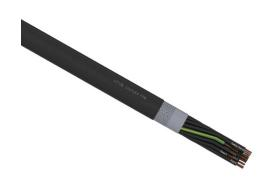
LUTZE Silflex FBP flexible control cable, shielded, 25 conductors (includes ground), 16 AWG, bare copper, polypropylene conductor insulation material, black with white numbers and green/yellow ground, TPE jacket, black, cut to length.
