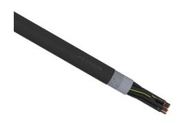
LUTZE Silflex FBP flexible control cable, shielded, 18 conductors (includes ground), 16 AWG, bare copper, polypropylene conductor insulation material, black with white numbers and green/yellow ground, TPE jacket, black, cut to length.
