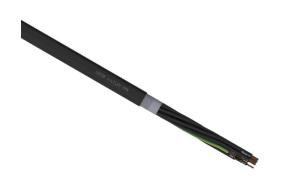
LUTZE Silflex FBP flexible control cable, shielded, 12 conductors (includes ground), 16 AWG, bare copper, polypropylene conductor insulation material, black with white numbers and green/yellow ground, TPE jacket, black, cut to length.
