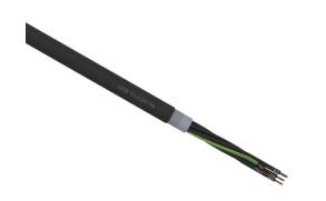
LUTZE Silflex FBP flexible control cable, shielded, 7 conductors (includes ground), 16 AWG, bare copper, polypropylene conductor insulation material, black with white numbers and green/yellow ground, TPE jacket, black, cut to length.
