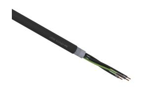
LUTZE Silflex FBP flexible control cable, shielded, 5 conductors (includes ground), 16 AWG, bare copper, polypropylene conductor insulation material, black with white numbers and green/yellow ground, TPE jacket, black, cut to length.
