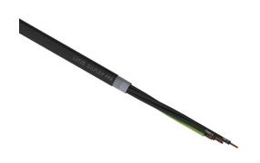
LUTZE Silflex FBP flexible control cable, shielded, 4 conductors (includes ground), 16 AWG, bare copper, polypropylene conductor insulation material, black with white numbers and green/yellow ground, TPE jacket, black, cut to length.
