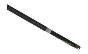
LUTZE Silflex FBP flexible control cable, shielded, 12 conductors (includes ground), 14 AWG, bare copper, polypropylene conductor insulation material, black with white numbers and green/yellow ground, TPE jacket, black, cut to length.
